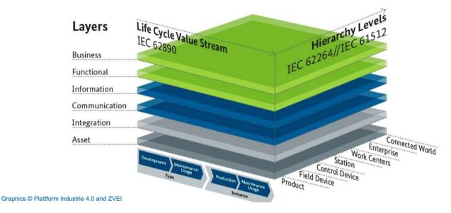
An Industry 4.0 reference architecture (RAMI 4.0) has been developed:
